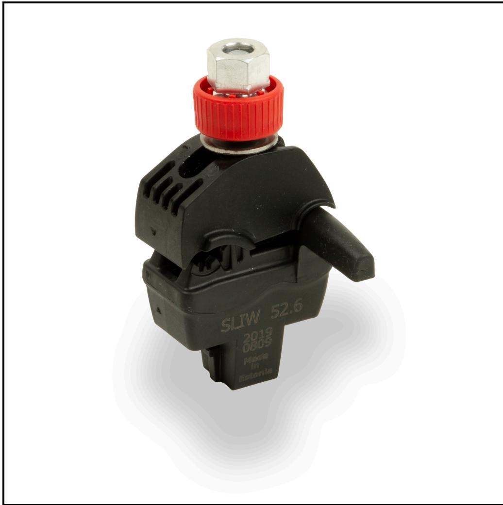
SLIW52.6 is for use with insulated aluminium or copper conductors. Fully insulated bolt provides safe live line working. Both main and branch conductor insulations are pierced by single bolt action. Test voltage 6 kV/50 Hz/1 min in water. Connector's design enables live line installation without peeling insulation from conductor.
